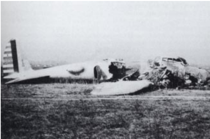
In 1935, just as it was about to win a big Army contract, the Model 299 crashed. The design was faultless—lack of a checklist doomed the airplane and some of the crew—but Boeing lost the contract, and the B-17 faced a five-year setback.
