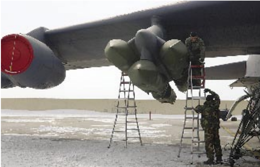
Airmen at Minot secure a mock missile to the pylon of a B-52H during an alert generation exercise.
