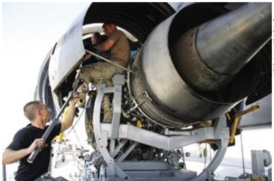
SSgt. Kevin Brown, SSgt. Joseph Dodson, and SSgt. Jamie Sherwood (l-r) install a replacement engine on a KC-10 Extender.
