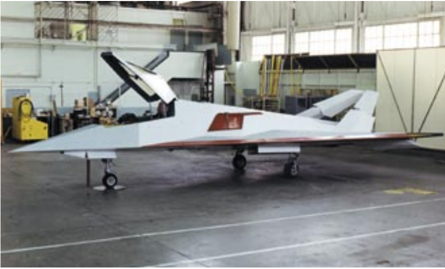
Have Blue, a low-signature, experimental, subsonic airplane powered by two J85-GE-4A engines, led to the development of the F-117.
