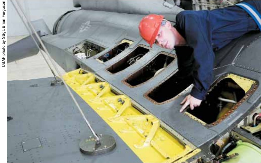
At Osan AB, South Korea, SrA. Malcolm Asher loosens a wing bolt on an F-16. The wing is being replaced due to corrosion and cracks found during routine inspection.
