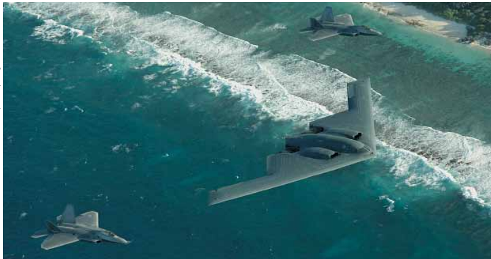
A brace of Raptors escorts a B-2 bomber off the coast of Guam. Peppered in with the legacy fleet, the limited number of F-22s will enhance USAF’s overall combat power.
